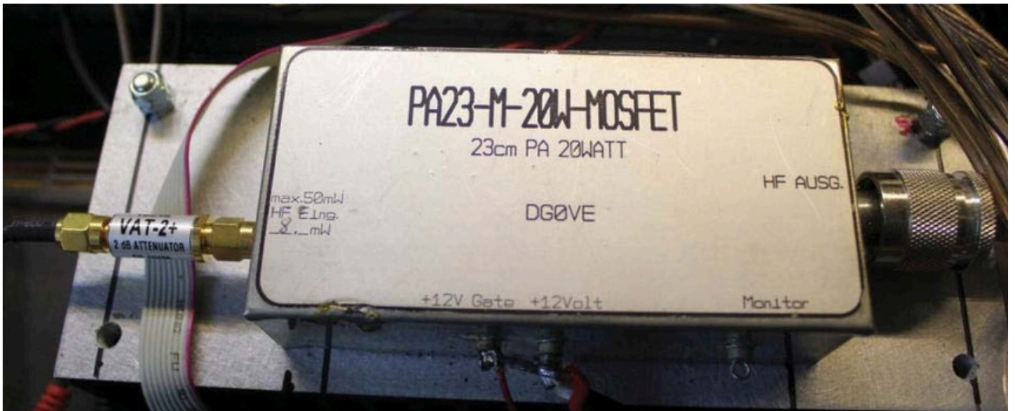
This transmitter has the DG0VE RA18H1213G 20 watt PA
